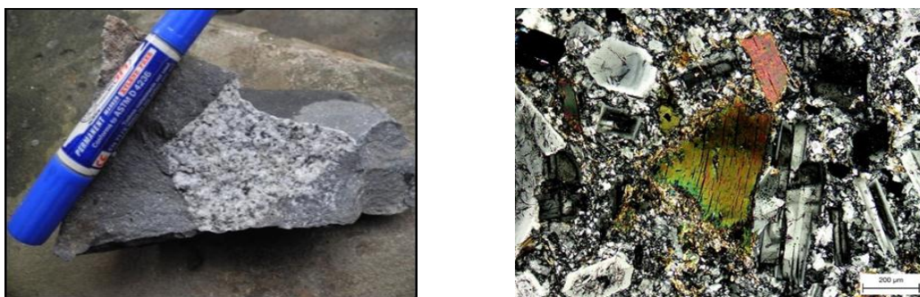
Figure 3 (a) Biotite granite xenolith in close-up view of camptonite lamprophyre (b) Showing strong pleochroism of subhedral biotite collected from Mokpalin and Kanni Quarries.
